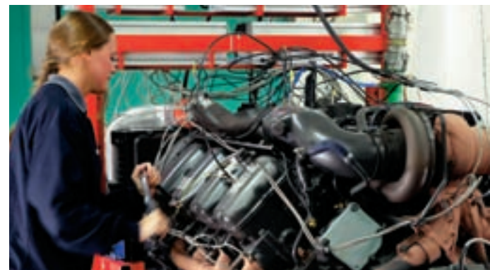
Scania has some 40 test cells, where engines are tested for performance and emissions.
