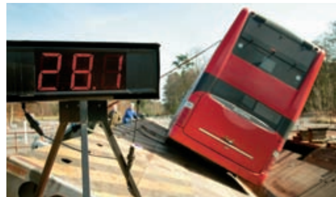
A Scania Omni double-decker undergoing rollover testing.
