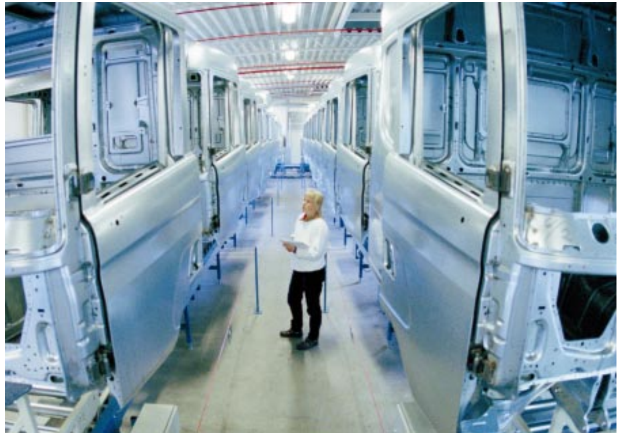
Unpainted cabs on their way in for priming at Scania's new paintshop in Oskarshamn, Sweden. Here all work takes place according to the Scania Production System.
